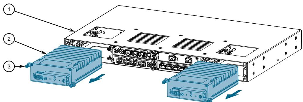
Figure 4.5 Removing a Power Supply
