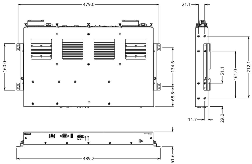
Figure 5.3 Panel and Din Rail Mount Dimensions
