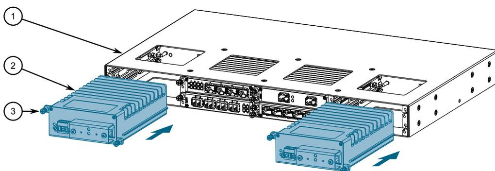
Figure 4.6 Installing a Power Module
