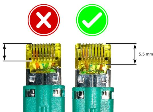
Adjusting the position of the connector in the port, either by wiggling or pulling the connector back, corrects the issue temporarily, but is not recommended. It may cause damage to the contact pins of the RJ45 ports. For a permanent solution, use Siemens 6XV1870-3Qxxx certified cables (manufactured December 2019 or after) or equivalent.
